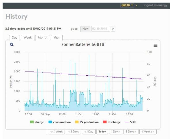
That 2% daily loss ends up being .2 kWh on the 10 kWh unit and .32 kWh on the 16 kWh unit. Over a year those losses equate to 116.8 kWhs & 73 kWhs. Sonnen is looking into other possible reasons for the high efficiency loss.
