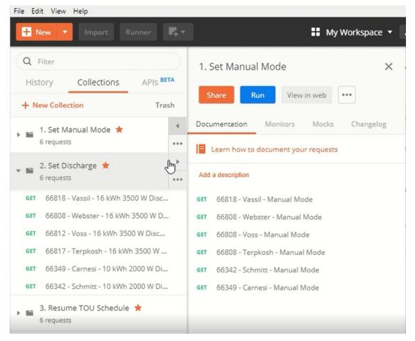
was all setup prior in order to make this process as seamless as possible. When you run this folder each of those commands will be sent and the units will start to discharge at those specific discharge rates.
