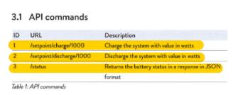
LAN. In order to have a smoother communication line and not have to continue to VPN into the homeowner's network, MiEnergy chose to go the direct URL command route. The API system allows server request URL command. This enables sending control commands through Sonnen's backend. Some of the URL commands include set discharge rate,
