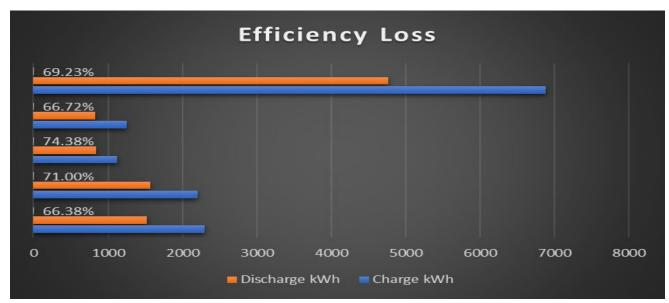
MiEnergy Cooperative used the total kWh that went to charge the battery unit, and then the total kWh that were discharged to calculate the efficiency loss. The numbers we found were much higher than initially expected. The efficiency in total was 69.23%. Keep in mind this loss is only on the battery unit. There would be extra loss from the two systems that have separate inverters
