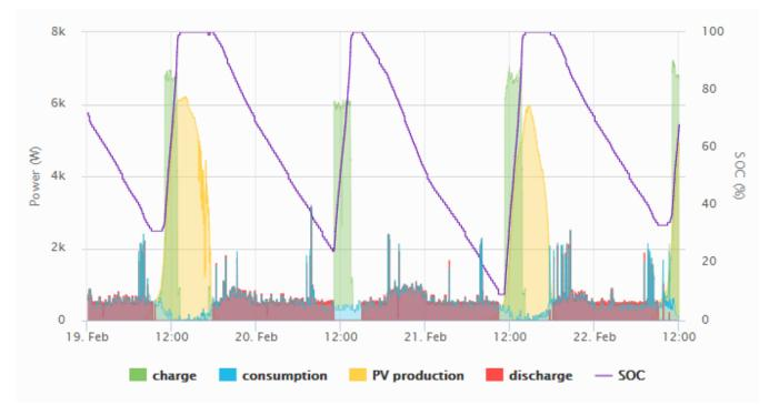
**-Yellow** is the PV production. In these TOU schedules the solar is designed to charge the unit. On February 20<sup>th</sup> it is visible that there was no solar production and on the 19<sup>th</sup> the solar charged the majority of the batteries.
